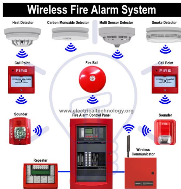
Figure 11: Wireless fire Alarm system (Electrical Technology 2019)
