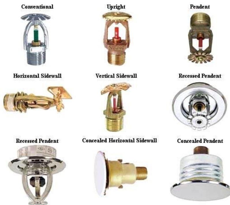
Fig. 12. Various types of sprinkler heads based on their application.
