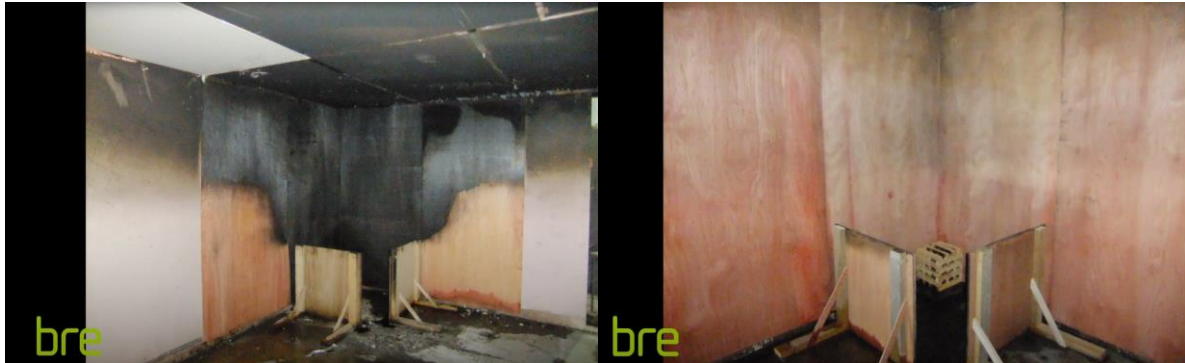
Fig. 14. Comparison of sprinkler application impact to fire development and spreading (BRE Group, 2013)
